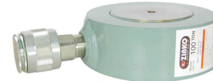
These ultra-high pressure low profile cylinders are perfect for any situation the requires a lightweight cylinder to fit where a lower pressure equivalent force unit cannot. The high pressure design allows the units to apply large amounts of force in tight places, perfect as a propeller positioning tool or for bearing press-in and extraction.
