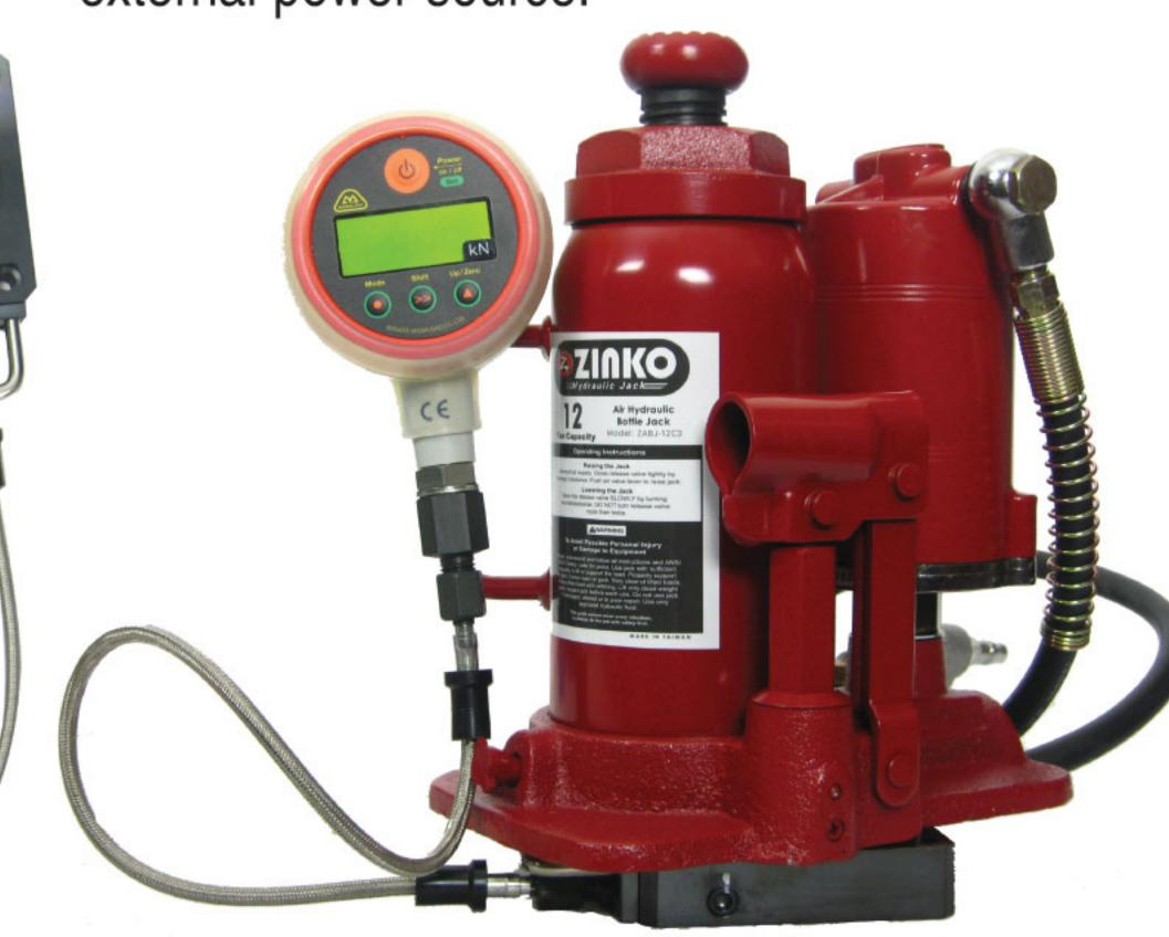
Air bottle jack on hydraulic load cell.
